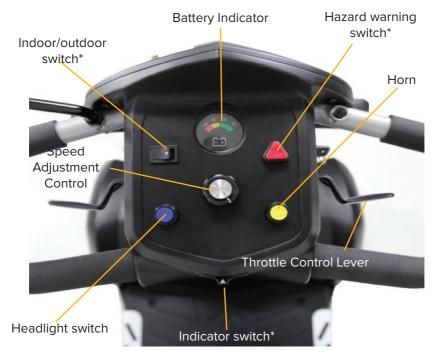
The above control panel is installed on the Envoy 6mph versions. The 4mph version does not include the switches marked with a "  $^{*}$ "
