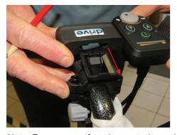
Slide the control panel onto the mounting bracket, until it clicks into position.
