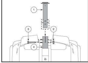
Figure 23. Seat Height Adjustment
