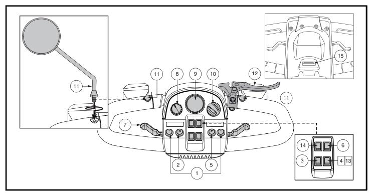
Figure 1. Tiller Console A
