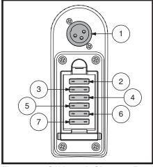
Figure 5. Off-board Charger Port/ Tiller Console Fuses
