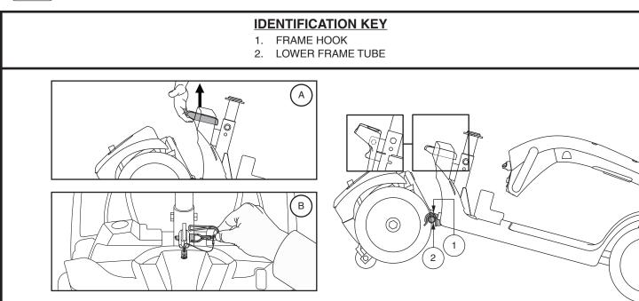
Figure 29. Frame Release Lever (Style A) and Frame Release Lockup Pin (Style B)
