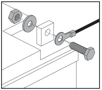
Figure 17. Battery Terminal Hardware - Configuration 1
