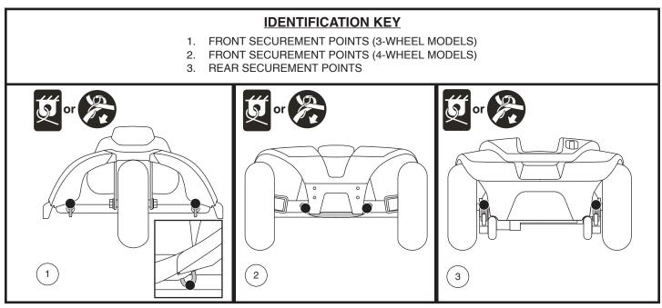
Figure 9. Securement Points (Identified with black dots)
