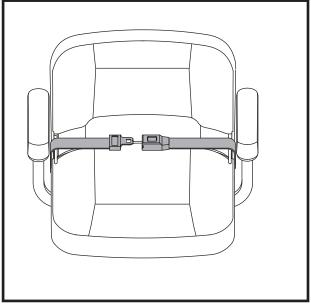
Figure 26. Positioning Belt - Metal Tab Style
