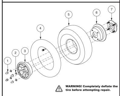
Figure 32. Pneumatic Drive Wheel Disassembly/Assembly
