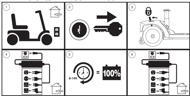
Figure 12. Battery Charging Procedures Diagram
