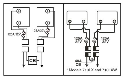
Figure 19. Battery Wiring Diagram
