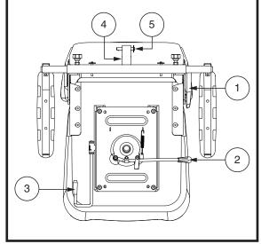
Figure 22. Seat Adjustments - Style B
