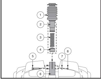
Figure 24. Seat Height Adjustment - Comfort Seat Post
