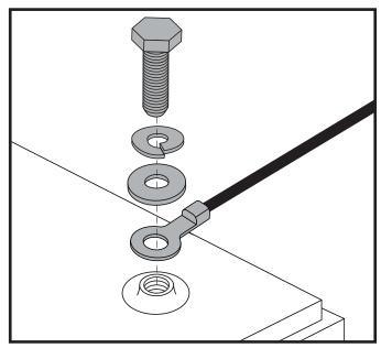
Figure 18. Battery Terminal Hardware - Configuration 2
