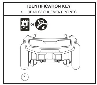
Figure 10. 710ZT - Securement Points (Identified with black dots)
