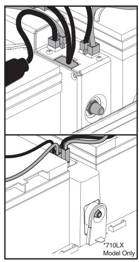
Figure 8. Main Circuit Breaker (Reset Button)
