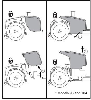
Figure 15. Battery Shroud Removal/Installation
