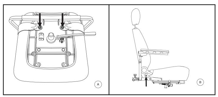
Figure 25. Positioning Belt Bolts
