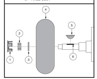
Figure 31. Wheel Removal
