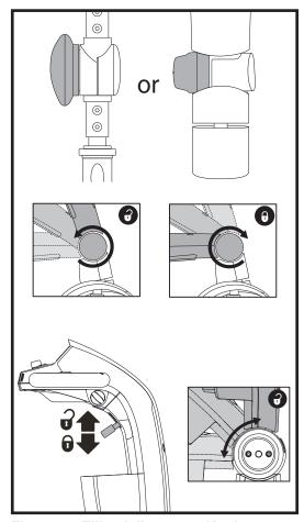
Figure 20. Tiller Adjustment Knob
