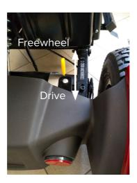
When the lever is pushed forwards, the scooter is in 'Freewheel' mode. The scooter motors and brakes are disengaged, and the scooter is free to move by hand.
