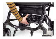
9. To insert battery. Slide the battery on to the rails underneath the seat. Push the battery firmly backwards until it locks in position with an audible click.
