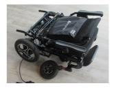
5. Unfold the powerchair. At the rear of the chair, set the right hand switch to 'I'. On the left hand switch, continually press the side marked 'II', until the powerchair is fully unfolded. Return the right hand switch to 'O'.
