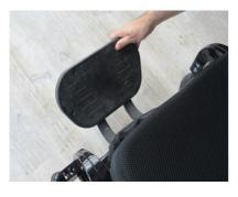
9. Install the seat and back cushions which attach with Velcro (if necessary)
