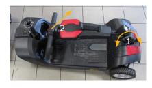
**3.** Connect the front and rear sections together. Hold the back of the rear section with one hand and lift the lever (3), on the front section, with the other. Hook the sections together and then release the lever, ensuring that they are securely locked together.
