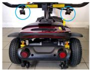
**9. Engage drive mode.** Ensure that the brakes are on and that the scooter is in 'Drive' mode, by pushing the freewheel lever backwards.
