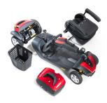
**2.** Raise the tiller on the front section. Turn the tiller adjustment knob (1) anticlockwise to loosen. Lift up the tiller (2) to the required position and then turn the tiller adjustment knob clockwise to secure.
