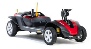
**6. Fit the seat.** Insert the shaft, under the seat, into the seat post on the scooter base. Lift up the lever (4) and rotate the seat gently, until it locks into position.
