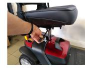
**7. Fit the basket.** Align the brackets on the basket with the brackets on the tiller and then press down to secure.
