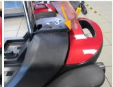
**4. Fit the seat post.** Remove the bolt from the seat post and then insert the post into the receiver in the scooter base. Insert the bolt and attach the nut. Secure the seat post using the hex key and spanner provided.
